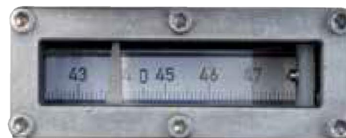
Level reading on graduated tape through window
